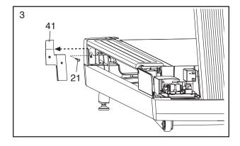
Remove the four indicated 1/4" x 3/4" Screws
