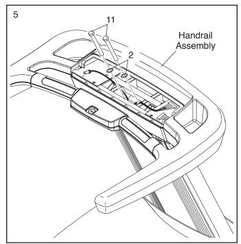
Tighten two 3/8" x 3 3/4" Screws (11) with two 3/8" Flat Washers (43) into the handrail assembly. Start both Screws, and then tighten them. See step 5. Tighten the two 3/8" x 3 3/4" Screws (11).
