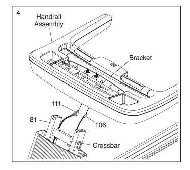
Attach the handrail assembly with two 3/8" x 3 3/4" Screws (11) and two 3/8" Star Washers (2). Start both Screws, but do not tighten them yet. Be careful not to pinch any wires.
