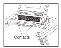
To measure your heart rate, stand on the foot rails and hold the contacts with your palms for approximately ten seconds; avoid moving your hands. When your pulse is detected, your heart rate will be shown. For the most accurate heart rate reading, continue to hold the contacts for about 15 seconds.
