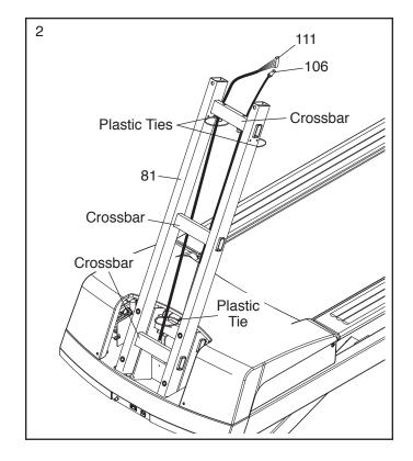
Slide the Upright Cover (80) downward onto the Upright (81). Be careful not to pinch the Upright Wire (111) or the TV Cable (106). Be careful not to hit your ceiling with the Upright Cover.
