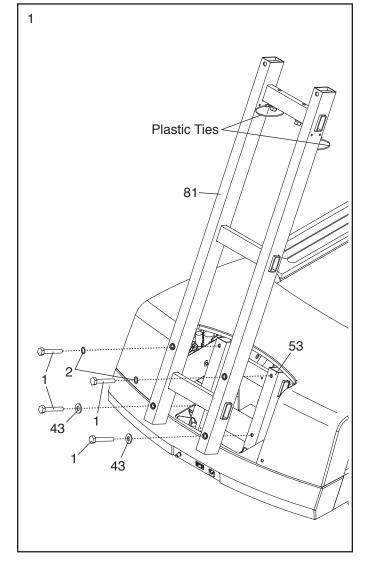
Insert the end of the Upright Wire (111) through the looped plastic tie at the top of the Upright (81). Make sure that the Upright Wire is behind the crossbars on the Upright. Then, gently pull upward on the Upright Wire as you tighten the plastic ties around the Upright Wire.
