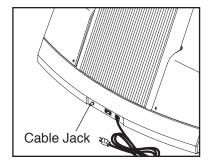
A satellite receiver, VCR, or DVD player can also be connected to the treadmill. Connect a CATV cable from the coaxial output on your equipment (usually labeled TV OUT or RF OUT) to the cable jack on the front of the treadmill.
